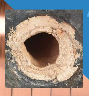
Mineral scaling is the established and recurring imbalance between water in the natural world and our modern built environments. Scale deposits typically go unnoticed until there is a crisis to resolve in a blocked pipe, repair or replace equipment, or now during the sustainability and energy movement to implement positive environmental changes.
