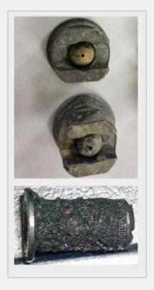
Screen and nozzle from the high pressure deburr machine. Maintenance would use acid cleaning to remove 12mm of calcium buildup in the nozzle
